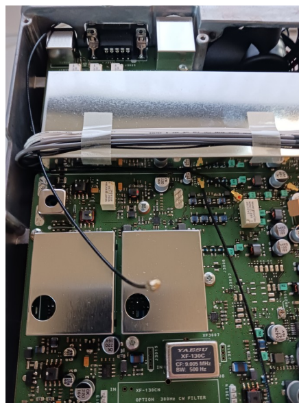
Figure.3 : U.FL to SMA cable installation.
