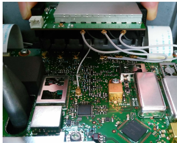
Figure.3 : Bypass cable connections.
