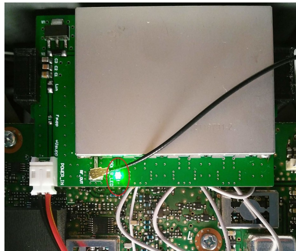
Figure.6 : Installed PTRX-9700 with power.
